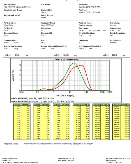
Figure 1 Particle Size Distribution Analysis on the Treated Effluent Sampled from Howe Sound Mill
